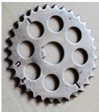
Figure 10: Four Stroke Timing Gear
